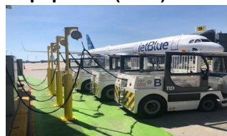
Figure 5-1. Example of Electric Ground Service Equipment (GSE)
