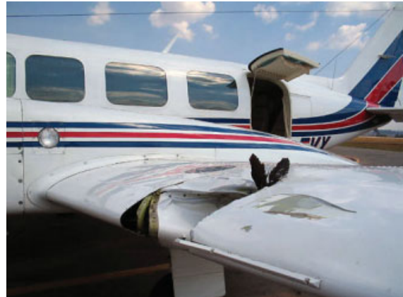
Figure 7 – Aircraft Wing Damage Due to Bird Strike
