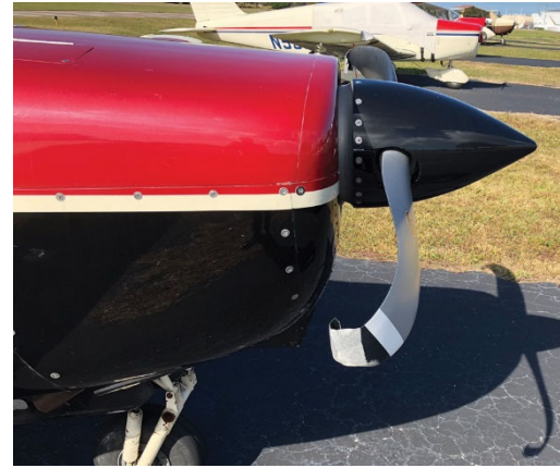
Figure 9 – Damage to an Aircraft After Prop Strike
