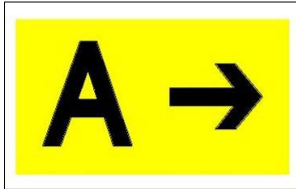
The sign is used to identify a taxiway
