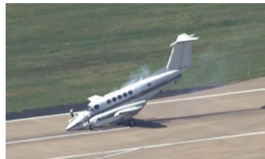
Figure 5 – Nose Landing Gear Collapse on Landing
