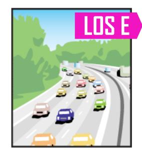
Unstable flow at or near capacity levels with poor levels of comfort and convenience.
