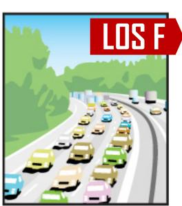
Forced traffic flow in which the amount of traffic approaching a point exceeds the amount that can be served. LOS F is characterized by stop-and-go waves, poor travel times, low comfort and convenience, and increased accident exposure.
