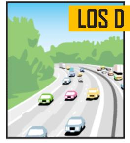
High-density flow in which speed and freedom to maneuver are severely restricted and comfort and convenience have declined even though flow remains stable.
