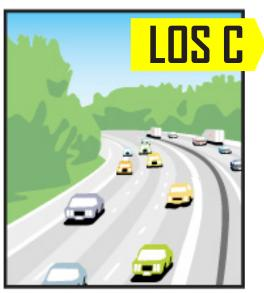
Restricted flow that remains stable but with significant interactions with others in the traffic stream. The general level of comfort and convenience declines noticeably at this level.
