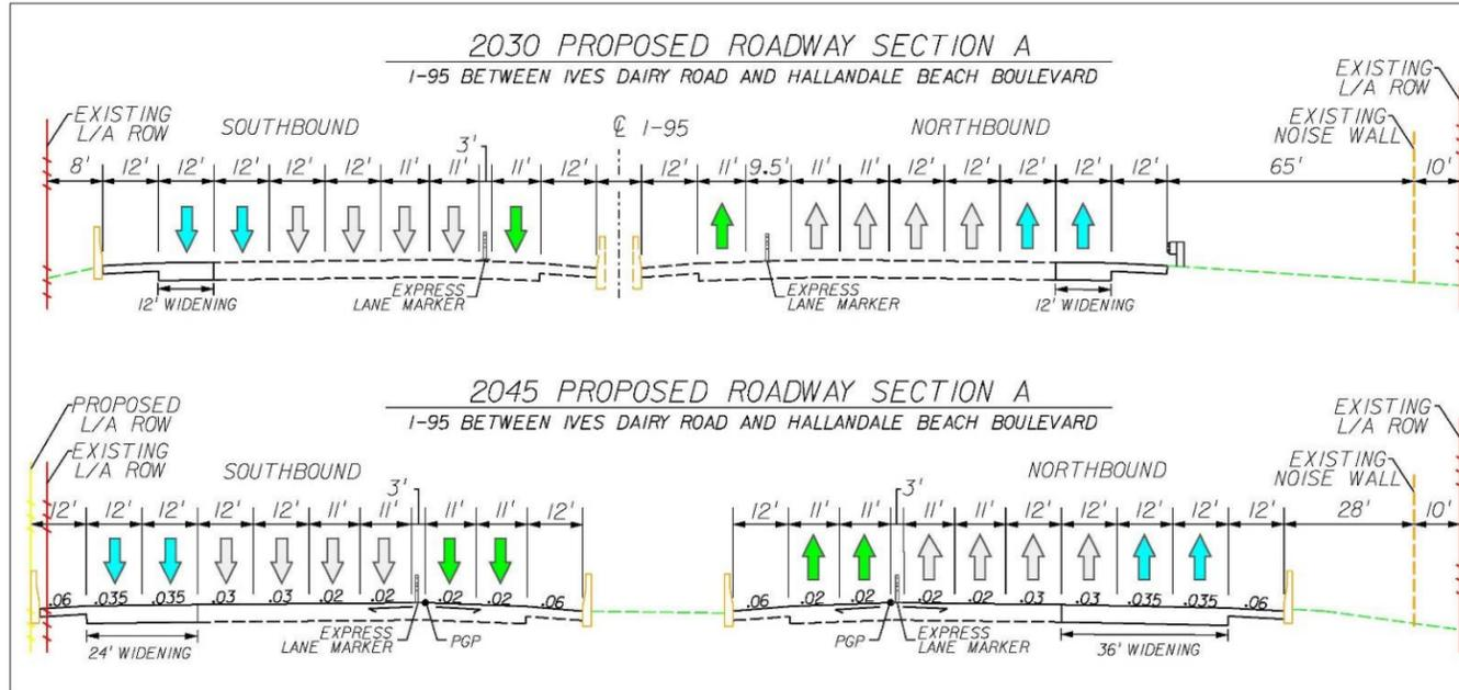
Figure 7.1 – Preferred Alternative Roadway Section A
