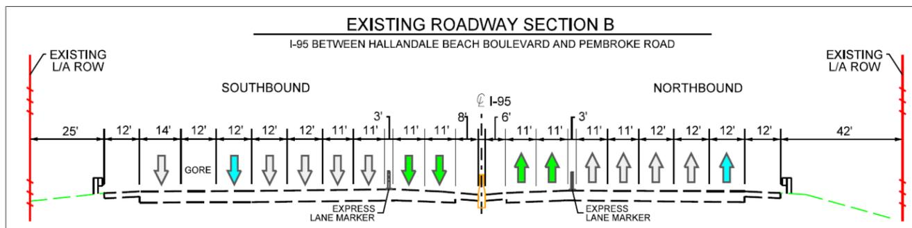
Figure 3.3 – Existing Roadway Section B
