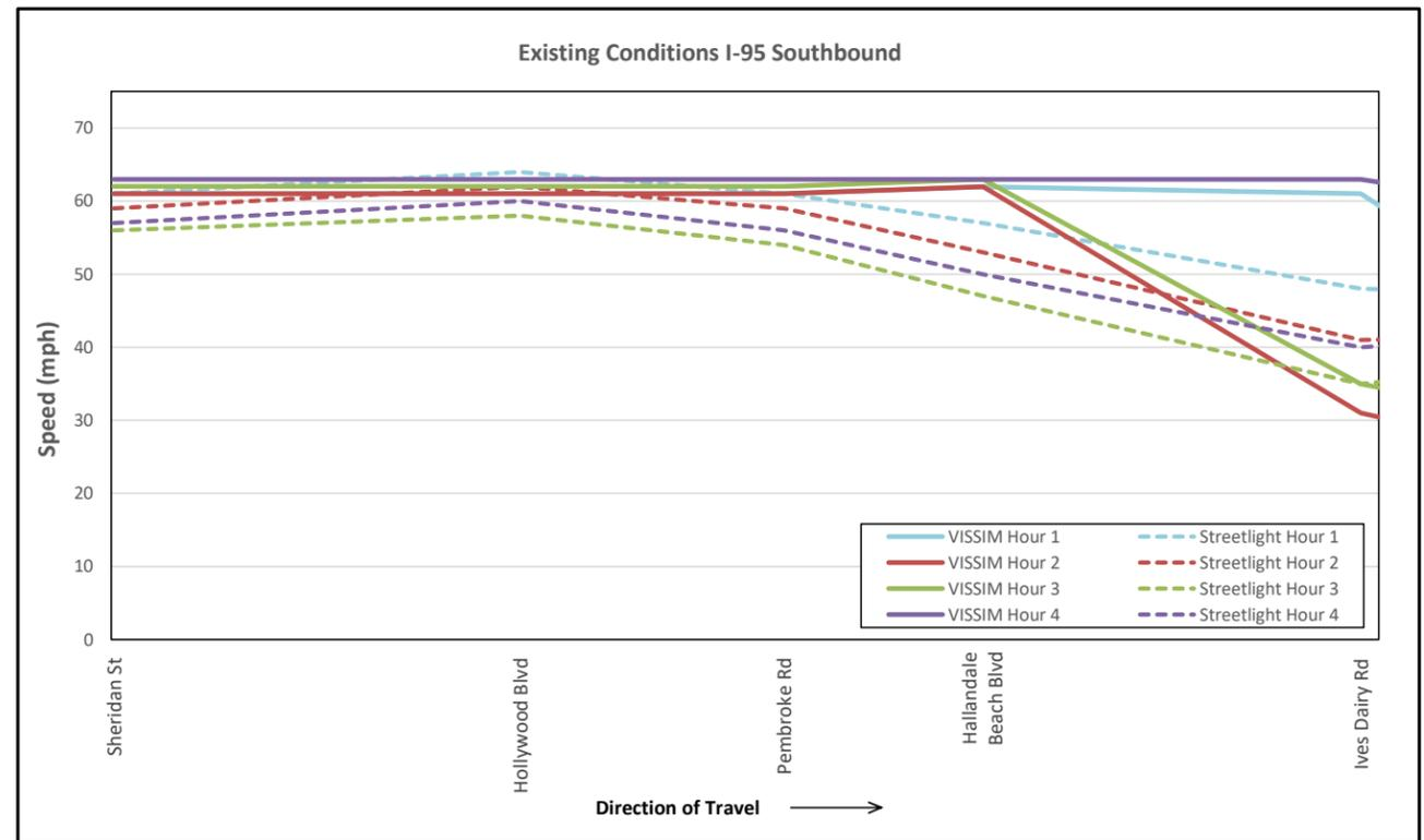
Figure 7.11: Existing Conditions Speed Profiles
