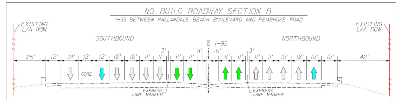
**Figure 5.7 – No-Build Alternative Roadway Section B**
