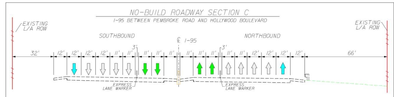
**Figure 5.8 – No-Build Alternative Roadway Section C**
