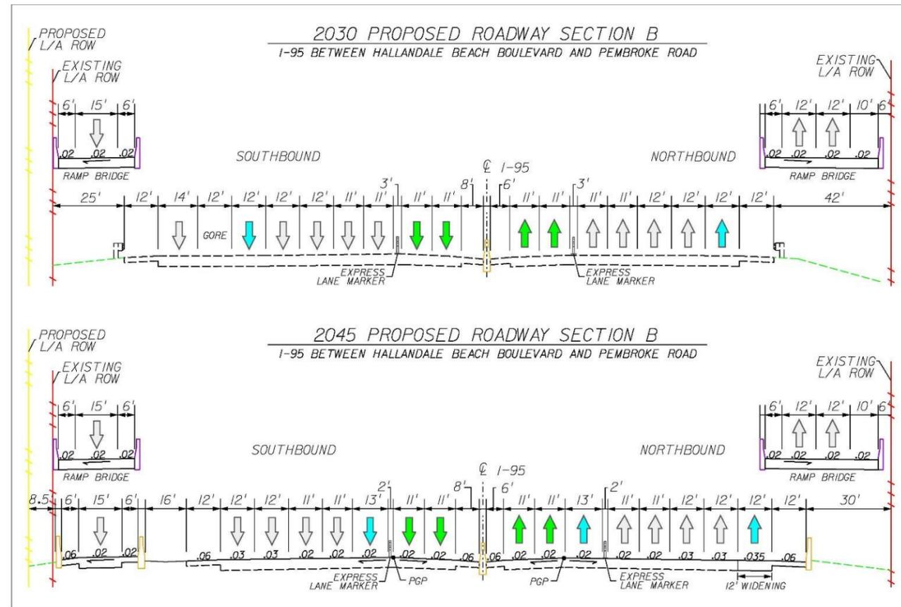
Figure 7.2 – Preferred Alternative Roadway Section B
