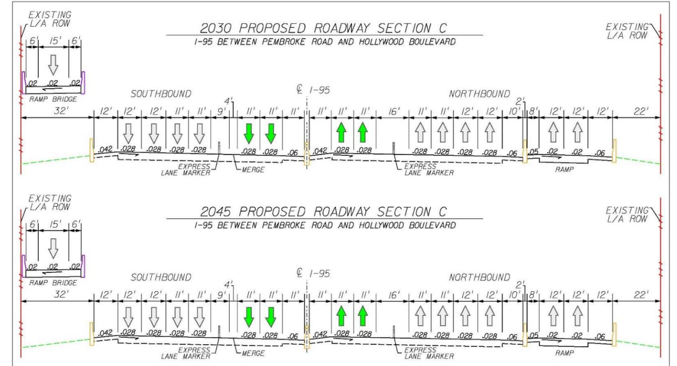
Figure 7.3 – Preferred Alternative Roadway Section C
