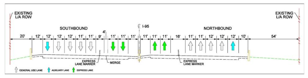
Figure 3.2 – I-95 No-Build Alternative Roadway Section North of Pembroke Road
