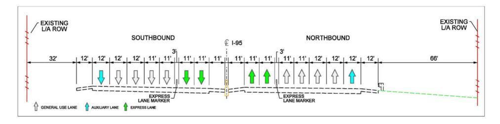
Figure 2.3 – I-95 Existing Roadway Section North of Pembroke Road
