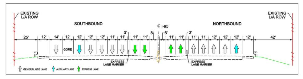
Figure 3.1 – I-95 No-Build Alternative Roadway Section North of Hallandale Beach Boulevard
