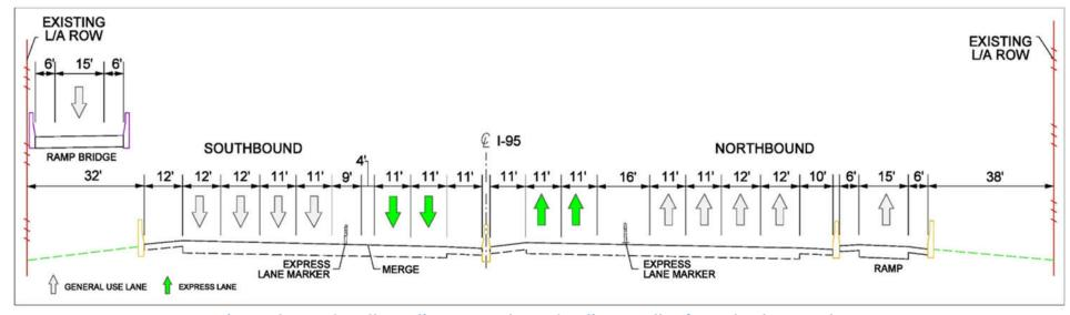
Figure 3.5 - I-95 Alternative 1 Roadway Section North of Pembroke Road
