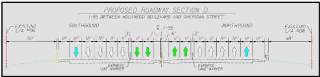
Figure 3.4 – I-95 between Hollywood Boulevard and Sheridan Street Existing and Proposed Cross Section
