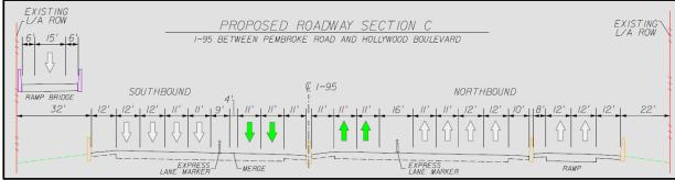
Figure 3.3 – I-95 between Pembroke Road and Hollywood Boulevard Existing and Proposed Cross Section
