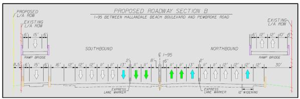
Figure 3.2 – I-95 between Hallandale Beach Boulevard and Pembroke Road Existing and Proposed Cross Section
