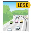
LOS D: High-density flow in which speed and freedom to maneuver are severely restricted and comfort and convenience have declined even though flow remains stable.
